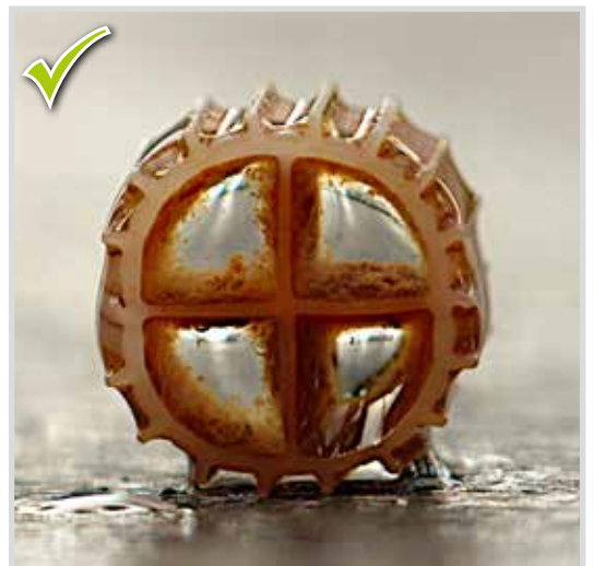
Bio-film on the filter materia
